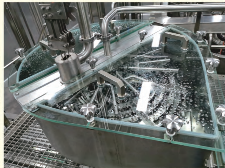
Caps lift to the disinfect and washing tunnel by the waterfall cap lifting system. After the soaking and jetting of sterile water, the caps was sent to the aseptic main filling machine for capping through the cap slide.
